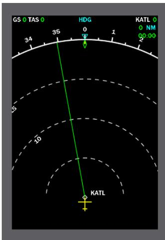
This is my FMC. It shows the standard view, with heading tape (lubber line) at the top, with range rings corresponding to the RANGE select slider on the main window.
